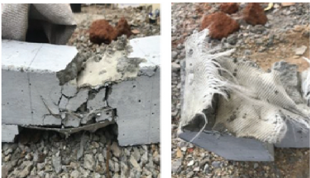
Figure 16. Beam Specimen after Failure due to Flexure Test Loading
