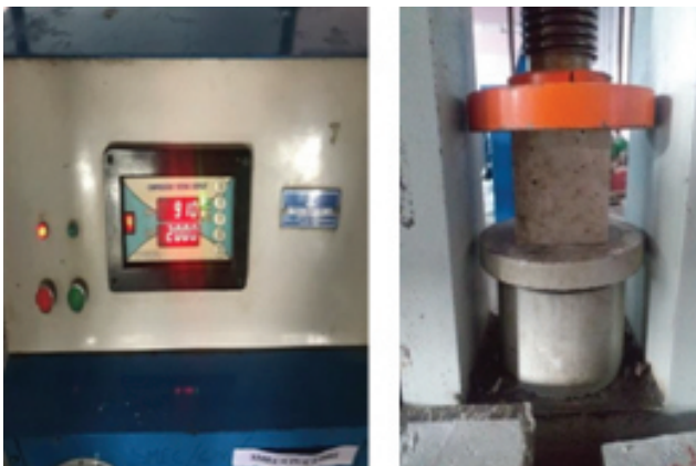
Figure 11. Compression Testing of Cube Specimen
