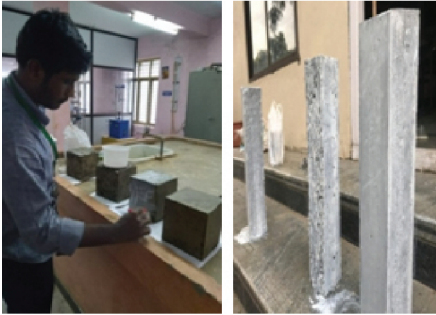
Figure 10. Application of Curing Compound for Hardened Concrete
