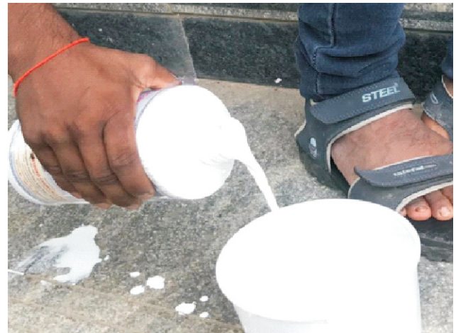
Figure 4. Curing Compound used for this Study
