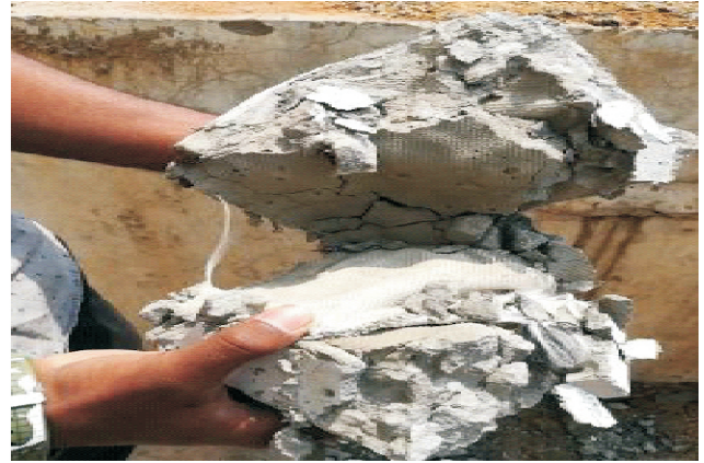
Figure 12. Cube Specimen after Failure by Compression
